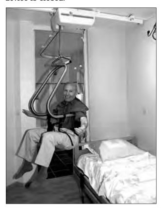
Move the lift into position so the swivel bar hook is over the center of the person's abdomen. Attach the web straps to the sling by placing the S-shaped hooks through the holes in the sling. Make sure the tips of the hooks point away from the person.
