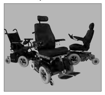
A main difference between models is the positioning of the larger, driving wheels that are coupled with two or four smaller wheels or casters to help balance and steer the chair. Consumers can choose from front- or rear-wheel drive systems, and the most recent innovation, a mid- or center-wheel drive wheelchair. Generally, the type of driving
